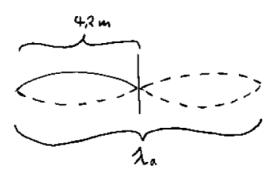
$$egin{aligned} \frac{\lambda_a}{2} &= 4.2 \, \mathrm{m} \quad \| \cdot 2 \\ \lambda_a &= 2 \cdot 4.2 \, \mathrm{m} \\ \lambda_a &= 8.4 \, \mathrm{m} \end{aligned}$$
